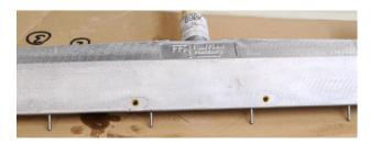
The pin squeegee must be set 1-2mm higher than the desired thickness of the elastic layer.
